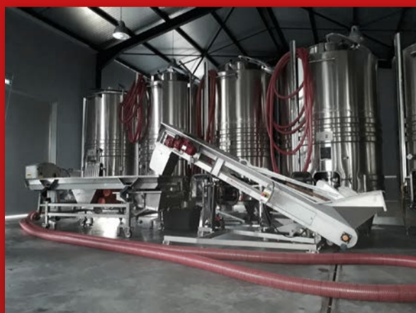
Grape selection lines, with automatic or manual sorting technologies
