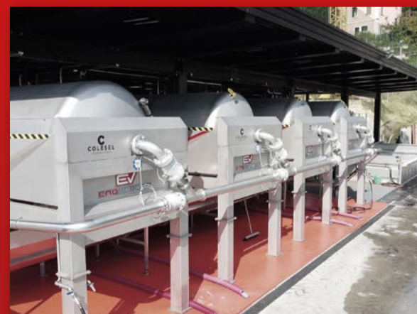
Pressing lines with continuous press system and remote control intergation
