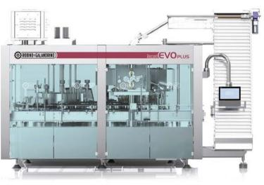
Wirehooder featuring bottle orientation (embossed logo on glass or glass mould seaming) prior the application of wirehoods achieving the desired position of the opening eyelet (via SNIPER vision
